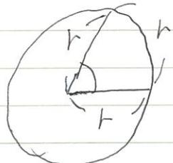
$$1 \text{ rad} = 57.29^\circ \quad - \text{② 弧の長さ} + (\pi / 3 \times 0.95)$$
